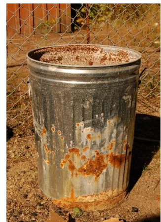
Ash stored in a corroded garbage can is unusable.
