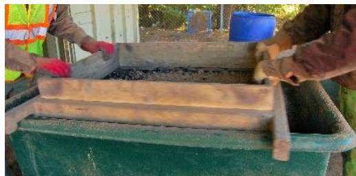
Handmade ash sifter being agitated over a poly box truck.
