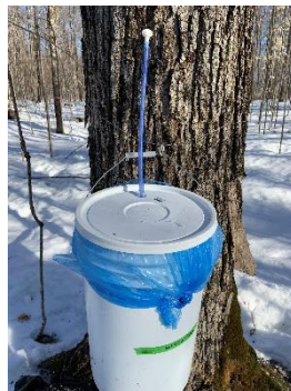
Apparatus taking sap from a sugar maple for sap flow assessment.
