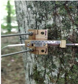
A tree fitted with a dendrometer
