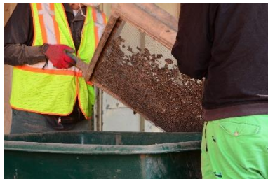
Handmade ash sifter being lifted to remove coarse char particles.
