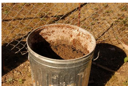
Ash stored in a galvanized garbage can that has gotten wet and become corroded.
