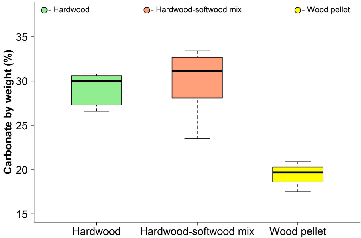
Figure 2.6. Box plots of carbonate by weight (%) in wood ash types. The box defines 50% of the observations with the median indicated by the thick horizontal bar. The whiskers delineate 95% of the observations.
